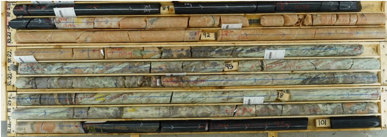
Figure 4: Pegmatite 1 as intersected in drill hole DDH22-09 at Raleigh Lake. Note the large microcline crystal immediately above the 6.5 metre interval (estimated true thickness based on structural measurements) of 40-50% spodumene mineralization.
